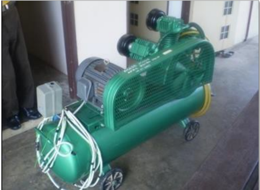
"Fu Sheng" 'CNS C4088' Triple Head Receiver Mounted Compressor, S/N 37B0600014, 1994, Taiwan, driven by "Teco" S/N 47121092, 5.5HP/4 Kw 3 Phase Induction Motor Air Compressor
