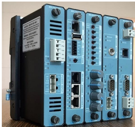
Figure 84: Remote Terminal Units (RTUs)
