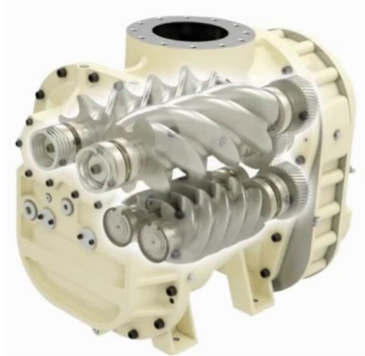
Figure 19: Rotary Air Compressor
